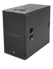
T212 delivers outstanding SPL in a compact form, featuring dual 12" neodymium woofers and a 1.4" titanium diaphragm driver. With switchable passive/bi-amp modes and a rotatable horn (60°×40° or 90°×50°), it offers flexible deployment and consistent directivity. Exceptional low-mid punch, smooth highs, and low distortion ensure natural, high-fidelity reproduction even at peak levels. Ideal for demanding applications requiring powerful output, wide coverage, and compact design.le.
